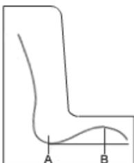
After production we can cut the foam to a specific inclination. Therefore we need the height difference between point A and B. Point A marks the lowest point in the seat, at the bottom. Point B marks the point at the lowest leg near the popliteal.
